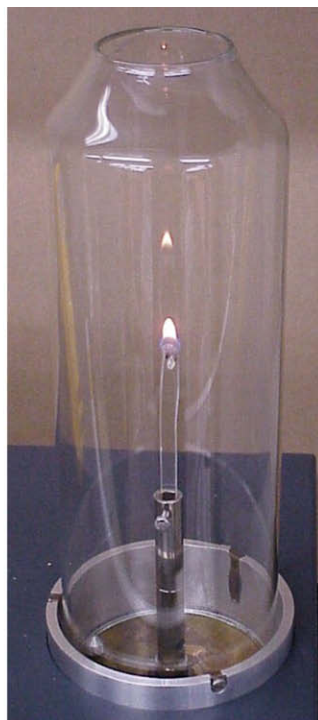
Fig. 24. Installation scheme and a photo of LOI test equipment [118].
